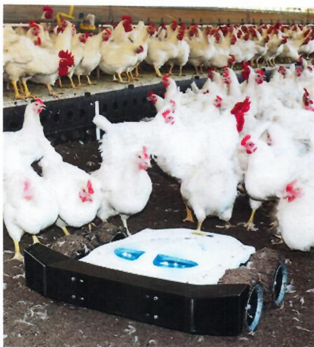
Tibot Technologies' Spoutnic Rover is an autonomous, wheeled robot that patrols the shed.
