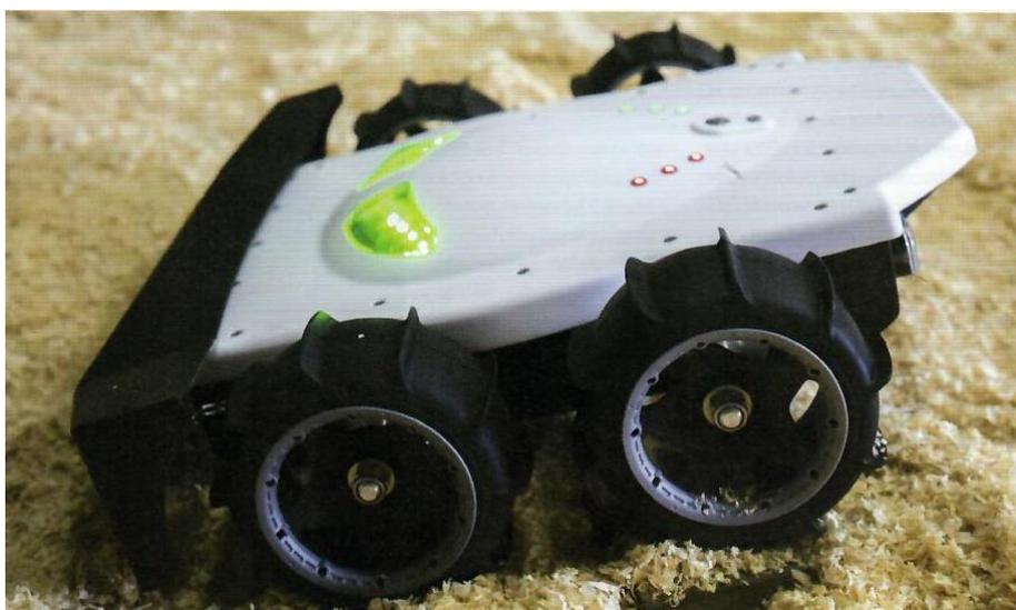
***Thanks to the Spoutnic robot, the forward speed (6 speeds possible), the light and sound stimuli (different colours and sounds) will stop the birds from getting used to the robot too quickly.***
